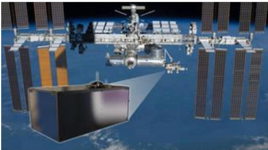
From its new vantage point on the International Space Station's Japanese Experiment Module - Exposed Facility, the Cosmic Ray Energetics and Mass (ISS-CREAM) mission, shown in the inset illustration, will study cosmic rays to determine their sources and acceleration mechanisms.
