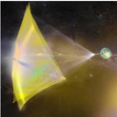
Artist's concept of Breakthrough Starshot nanostarship. A 100-gigawatt light beam to propel approximately 1,000 ultra-lightweight nanocraft like this one to 20 percent of light speed. This fleet of nanostarships could reach the three stars of the Alpha Centauri system within about 20 years of launch. Image via [BreakthroughInitiatives.org](http://BreakthroughInitiatives.org).
