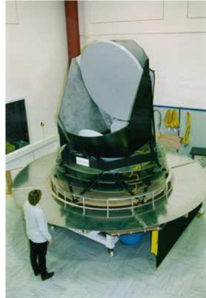
The information Planck has to gather lies in the pattern formed by these slightly hotter and colder regions, called 'anisotropies' or 'inhomogeneities'. As a consequence, the Planck detectors will have to be highly sensitive and will have to work at temperatures very close to the absolute zero, otherwise their own emission of heat will spoil the measurements.
