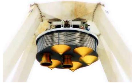
The RF receiver package after installation on the antenna, showing the solar shield as well as the scattering cones that were installed in the place of the five non-fitted receivers.
