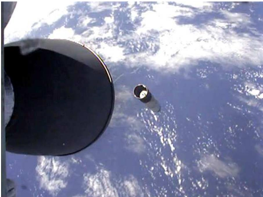
The critical stage separation sequence began about 2 minutes and 37 seconds into flight with shutdown of the Merlin first stage engine, then separation of the first and second stages, followed by ignition of the Kestrel second stage engine. Photo © 2008 Space Exploration Technologies Corp.
